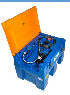
The TPDU-P features the same convenience, portability, and durability of the TPDU-M, but in a slightly lighter weight package. Made from ISO 22241 compliant rotationally molded high density polyethylene (HDPE,) the PDU-P is UV and rust resistant for years of service in the harshest of conditions. The TPDU-P is equipped with our TD10-12V diaphragm pump.
